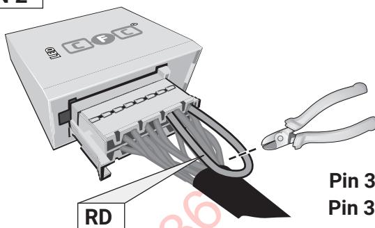
Pin 3 and Pin 2 disconnected
