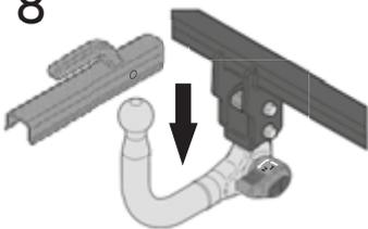
✓ Each time you install the towball into the socket, you must ensure that you can see the green field on the towball handle (3) and apply additional physical force to ensure that the towball is securely fastened in the socket. (6)
