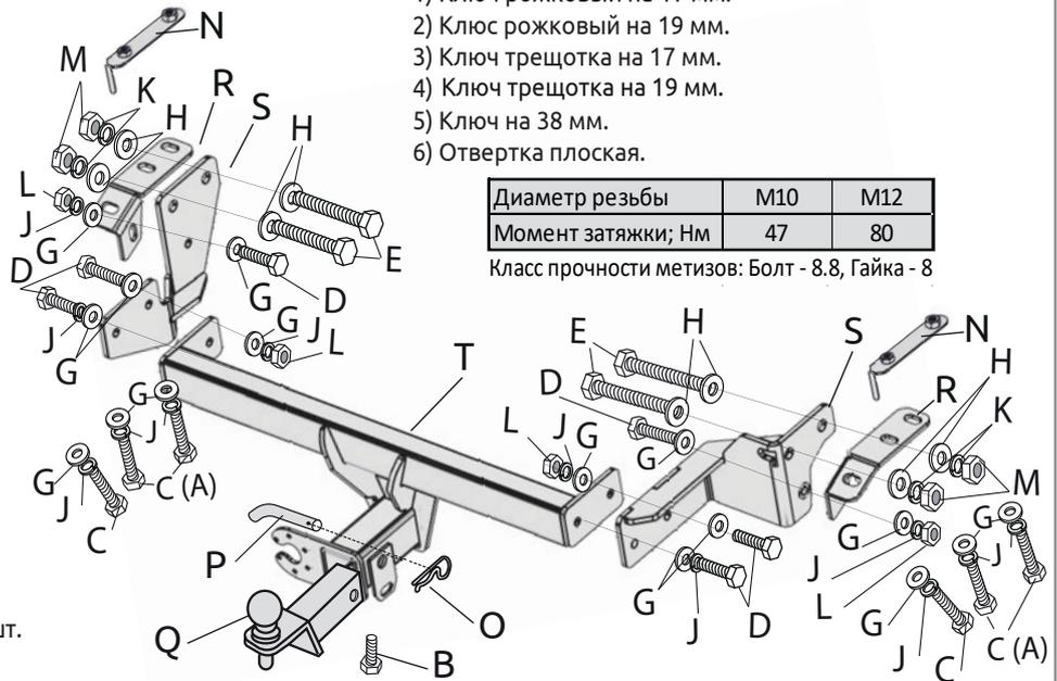
Table with 3 columns: Диаметр резьбы, Момент затяжки, Нм, and Class of strength. Values: M10, M12, 47, 80.
